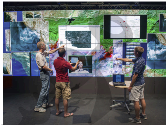
Fig. 1. An example of 4 live video streams on a 32 screen tiled display wall. Researchers and a remote collaborator compare a collection of images from previous San Diego County fires with video streams of a real-time wind flow visualization, current fire locations map on a tablet, and live panoramic images from various San Diego County locations on a laptop.
