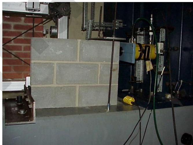
Figure 4. In-plane, destructive shear test set-up.
