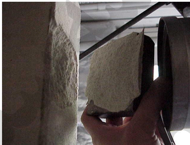
Figure 26. Plate separation from AAC wall panel during AACT3.
