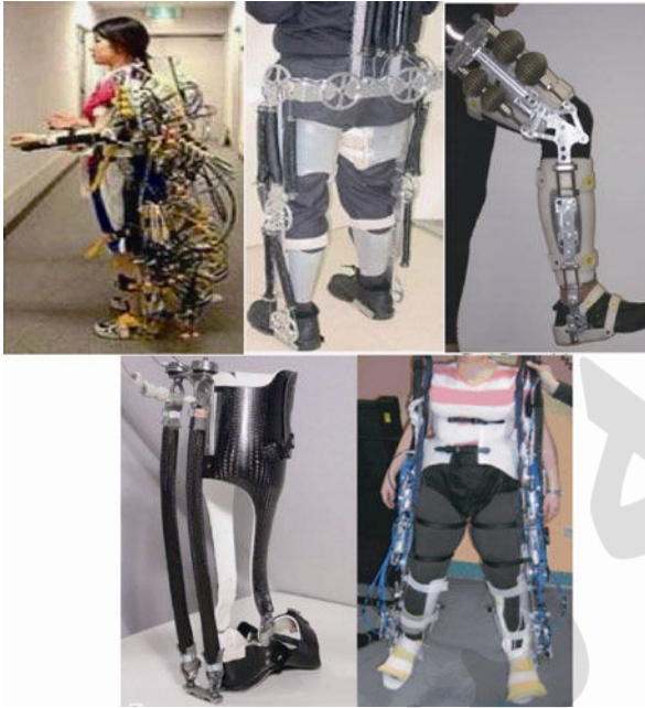
Fig. 6. Experimental devices driven by pneumatic system
