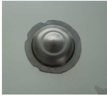
Figure 6: Final sheet part produced with ISF on CNC lathe machine
