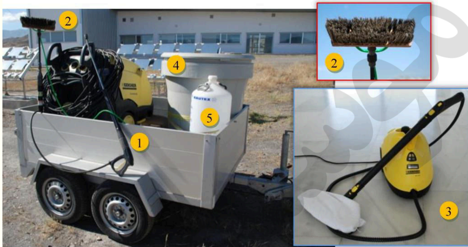
Fig. 4. Pressure washing device with hand spray nozzle accessory (1), water-fed natural horse-hair bristle brush accessory (2), steam cleaner (3), demineralized water tank (4), and additives tank (5).
