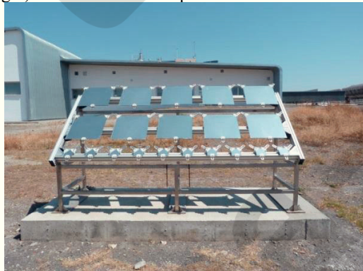
Fig. 2. Structure 2 (left) and distribution of solar reflectors per type in a test bench (right).
