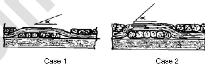
Fig. 6. Comparison between low and high packing in aramid braid (Bryant, 1990).
