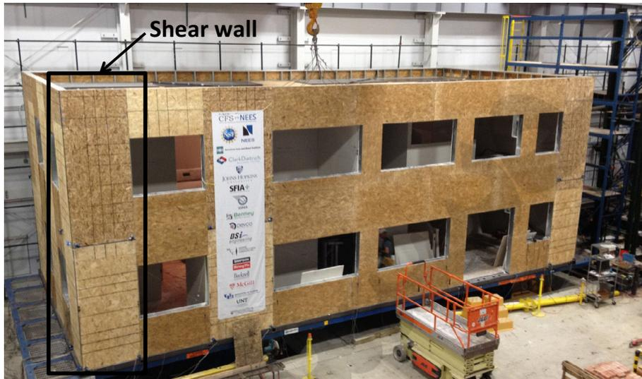
Fig. 1. CFS-NEES building and shear wall in it.
